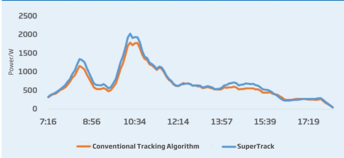
up to 35% and a power generation gain of up to 4.64%. In typical overcast conditions, the conventional tracking algorithm rotates at an angle to the sun, resulting in a lower output, while the SuperTrack array rotates to a smaller angle, resulting in an overall power gain of 9.41%.
