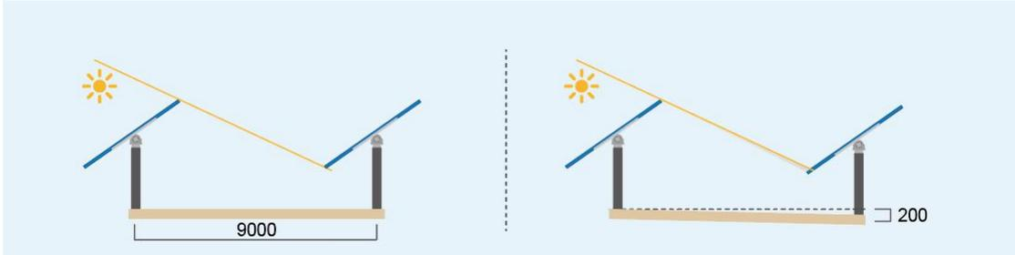
At the same time, due to different terrains between arrays, if shade is caused in the morning, light leakage may be found at the stage of backtracking in the afternoon, thereby leading to inadequate utilization of resources. (Figure 6)
