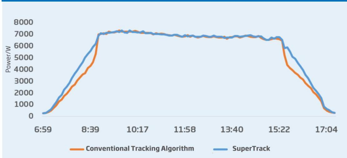
(Note: The gain comparison is for single-row tracker which are shaded in both the morning and afternoon)
