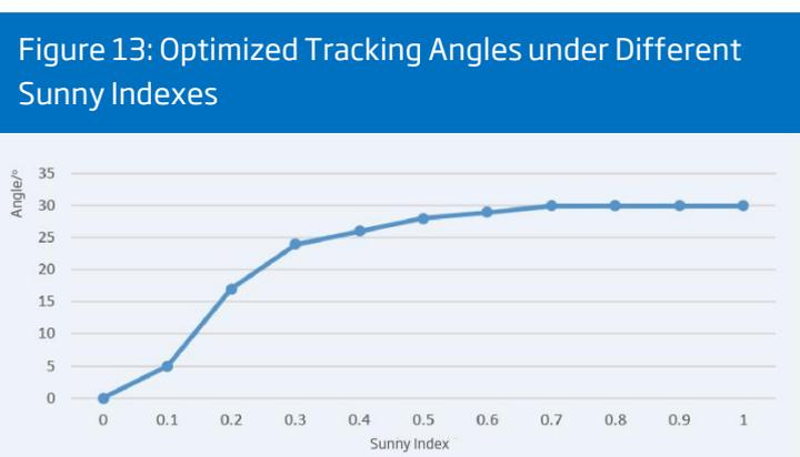
Based on the BIM, the tracking angles are different under different weather states. Specifically, sunny index (0-1) is defined different weather states, the higher the sunny index
