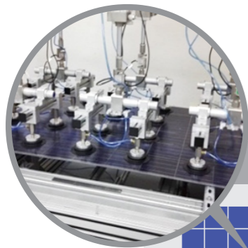
Regular framed module Deformation @ 31mm
